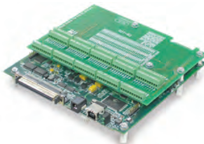
DaqBoard/3001USB with TB-101 screw-terminal board attached
